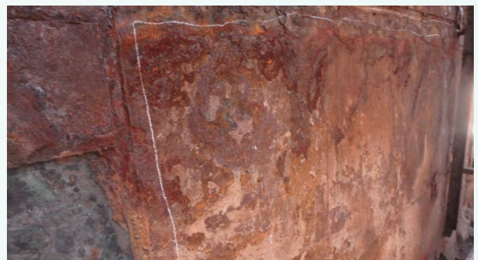
Corroded ESP casing
