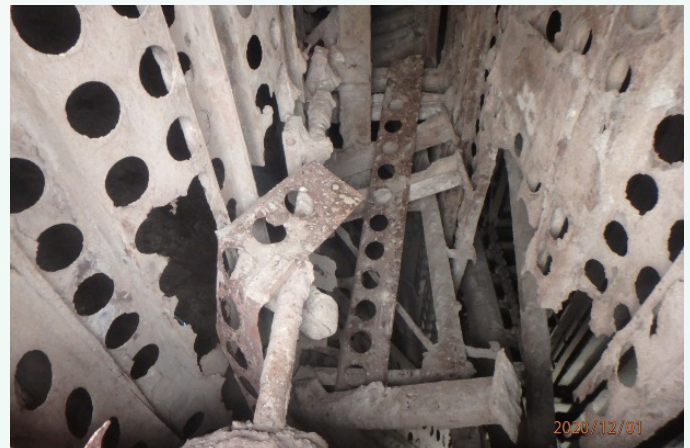
Severely damaged Gas Distribution (GD) screen
